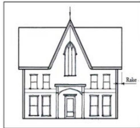
Rake is the amount that the gable end of the roof extends beyond the wall on that end of the structure.
