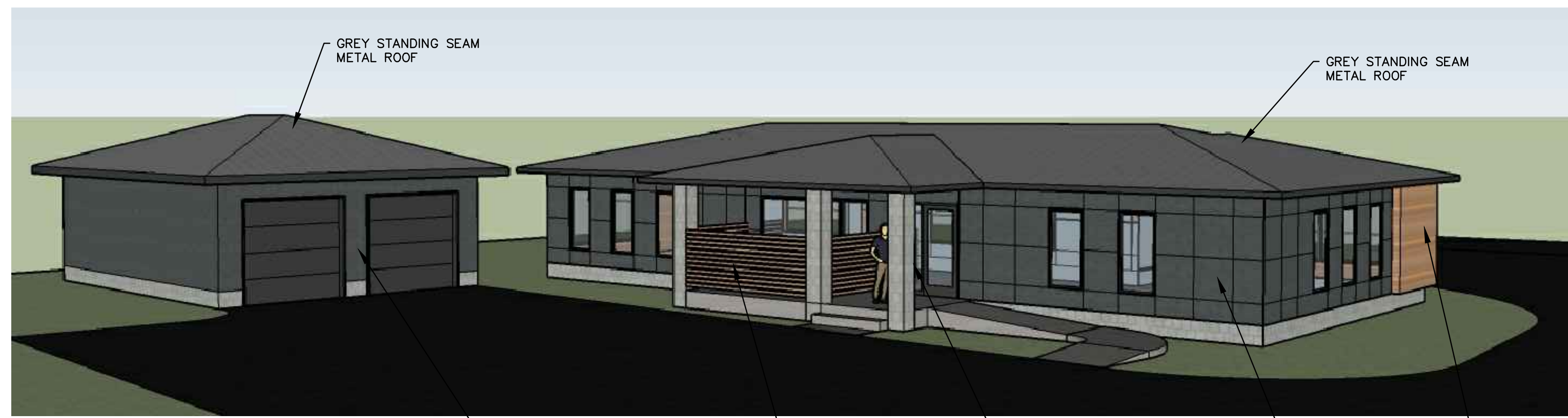
E SOUTH ELEVATION (MAIN ENTRY) SCALE 1/4" = 1'-0" Labels: GREY STANDING SEAM METAL ROOF, GREY CEMENT BOARD, WOOD LOOK CEMENT BOARD SCREEN WALL, SPLIT FACE CMU COLUMNS, GREY CEMENT BOARD, WOOD LOOK CEMENT BOARD
