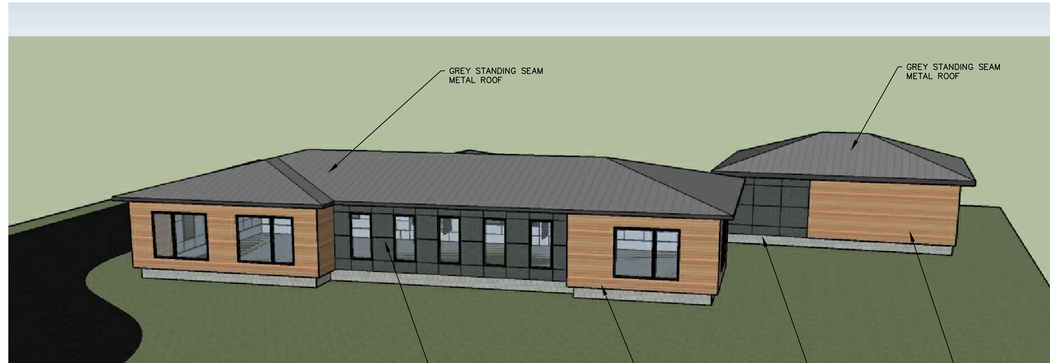
E NORTH ELEVATION (FACING ROAD) SCALE 1/4" = 1'-0" Labels: GREY STANDING SEAM METAL ROOF, GREY CEMENT BOARD, WOOD LOOK CEMENT BOARD
