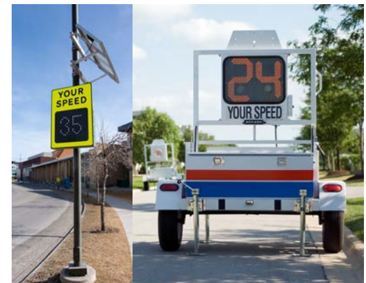
Speed monitoring signs and increased enforcement are effective traffic calming methods
