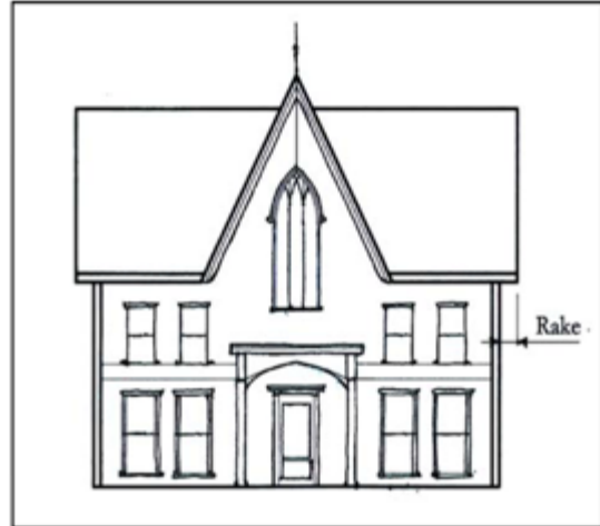
Rake is the amount that the gable end of the roof extends beyond the wall on that end of the structure.
