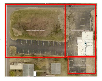
The proposed site access plan includes a total of two points of ingress and egress, one located on Mosel Avenue and the other located on Woodward Avenue. Both ingress/egress points are approximately 31 ft. wide. The parking plan includes 39 parking spaces located primarily on the eastern portion of the site. The applicant is proposing to remove the existing asphalt and concrete areas located on the site.
